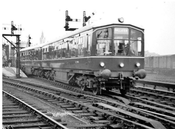
Figure 9: View of the BR Scottish Region battery-electric multiple unit departing from Aberdeen on its first day of passenger-carrying service on the Aberdeen – Ballater line (April 1958). The compartments holding the lead-acid batteries are visible below the body of each of the vehicles of the two-car set. (Photograph D. Murray-Smith).
