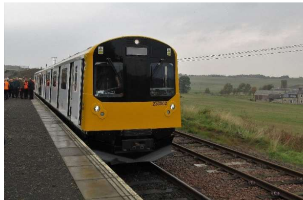
Figure 8: The Vivarail Class 230 battery-electric unit at Manuel prior to departure for Bo'ness (Photograph D. Murray-Smith).
